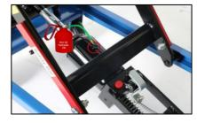
5. Release the Control Lever, and pump slowly to raise the Table to its full height.
